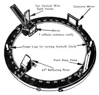
THE PURPOSE OF THIS GTA IS TO SHOW YOU THE BASIC STEPS REQUIRED FOR TAKING A FIX USING AN AZIMUTH CIRCLE.
