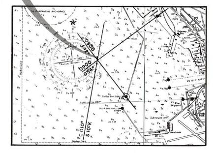
The fix is established at the point where two bearing lines cross. The greater the angle between the two bearing lines, the more accurate the fix.
