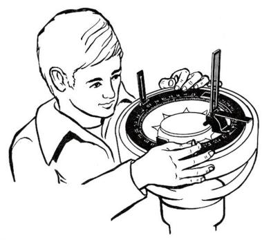
6 When the object is lined up with the two sight vanes, take the bearing reading that is reflected in the mirror located under the far vertical wire sight vane. Record the bearing and time.
